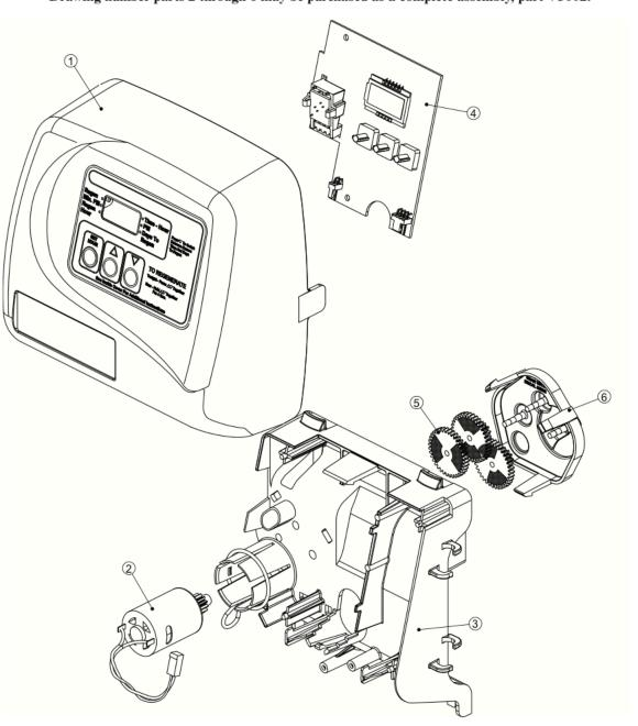
WS1TC Drive Cap Assembly, Downflow Piston, Regenerant Piston and Spacer Stack Assembly
